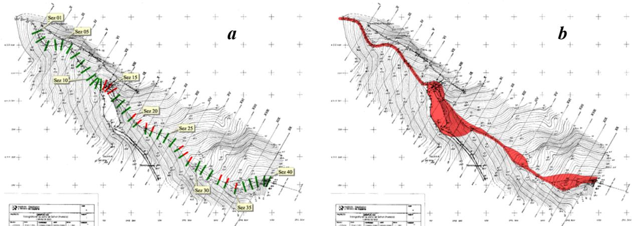
Figure 9.- (a) Cross sections along the Sahún fan channel. The red ones indicate total overflow, the red and green ones indicate lateral overflow. (b) Debris flow affected areas
