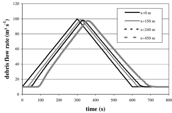
Figure 6 – Debris flow routing trough a rectangular channel 450 m long ( $C^* = 3$ ;  $S = 19\%$ ; width  $B = 5$  m; abrupt narrowing to  $B = 3$  m from  $x = 210$  m to  $x = 240$  m): *flow rates hydrographs*
