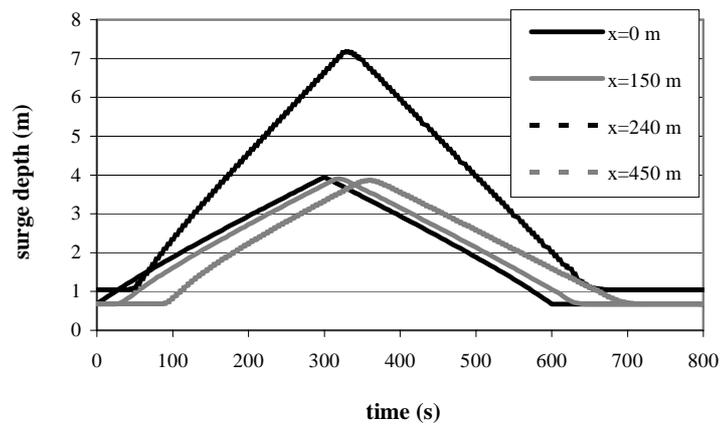
Fig. 7 – Debris flow routing trough a rectangular channel (same conditions of figure 6): *surge depths hydrographs*
