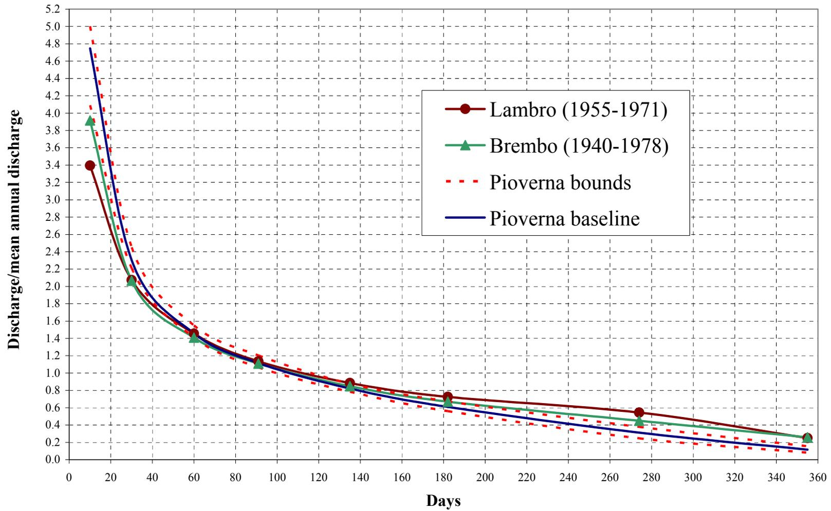
**Fig. 3 Comparison of the normalized flow duration curves measured for the Lambro and Brembo rivers with the simulated baseline curve and uncertainty bounds for the Pioverna at Bellano**
