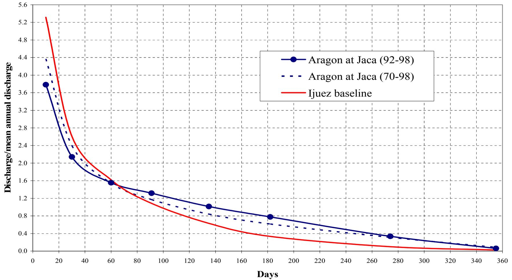
**Fig. 6 Comparison of the normalized flow duration curve for the scaled Aragón discharge record at Jaca with the simulated baseline curve for the Ijuez outlet**
