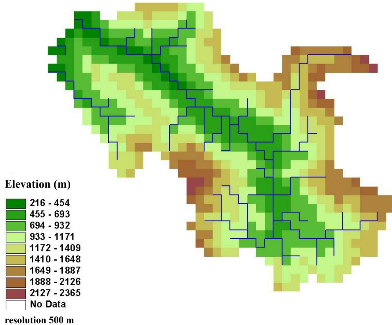
**Fig. 1 SHETRAN grid system, channel network and elevation distribution for the Pioverna and Esino focus area**
