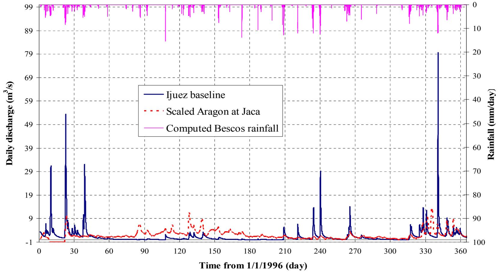
**Fig. 5 Comparison of the simulated baseline daily discharge for the Ijuez outlet with the scaled discharge for the Aragón river at Jaca for 1996. Also shown is the rainfall record derived for Bescos in the Ijuez catchment**
