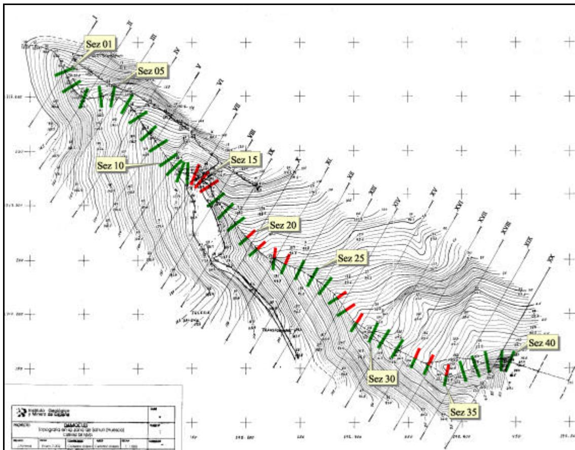
**Figure 3 – 1-D MODDS output simulation carried out hypothesising 197 m<sup>3</sup>/s of maximum debris-flow discharge and re-entering overflow solid material from first bridge. Red colour individualises overflow sections.**
