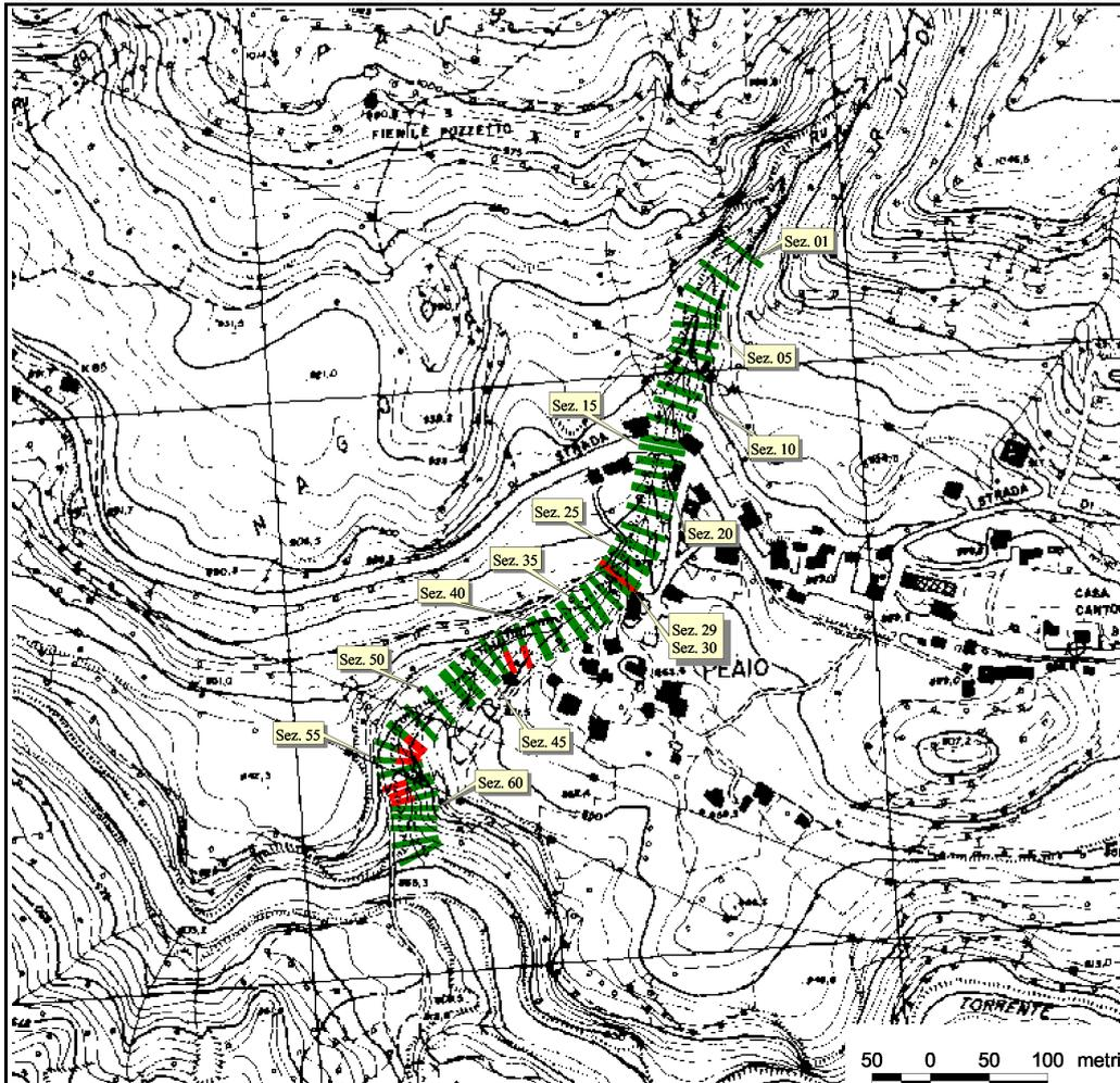
Figure 9 – 1-D MODDS output. Red colour individualize overflow sections.
